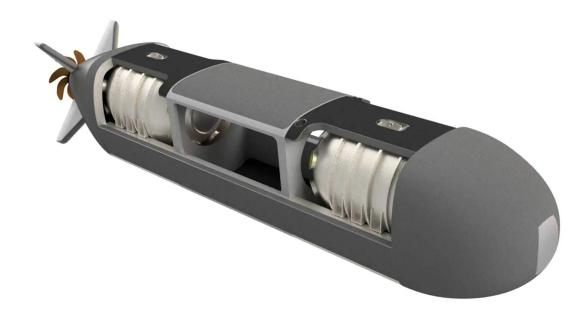
CETUS is a modular XLUUV featuring two pressure vessels separated by a central (flooding) payload bay.
