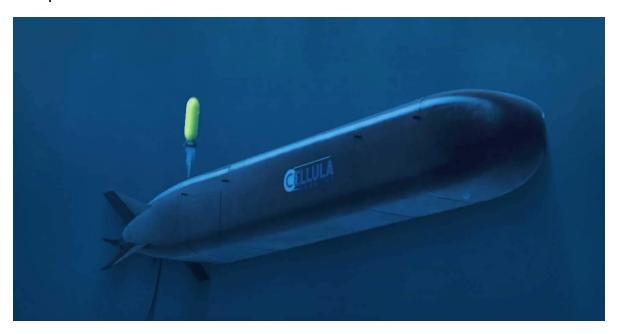
The Canadian Cellula Solus XR-2 is powered by hydrogen fuel cells providing a submerged range of over 5,000 km at 3 knots. It was designed with under-ice operations in the Arctic in mind (CGI: Cellula).
